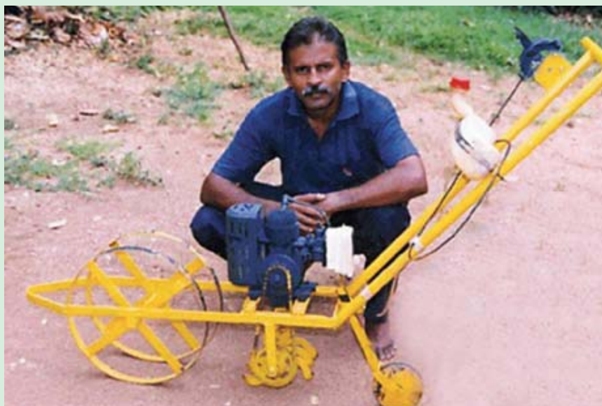
Motorized weeder developed by S. Ariyaratna, Sri Lanka.
