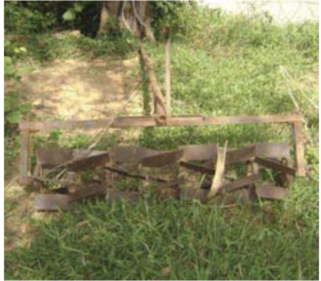
A bullock drawn puddler used for SRI. It does not disturb the land levelling.
