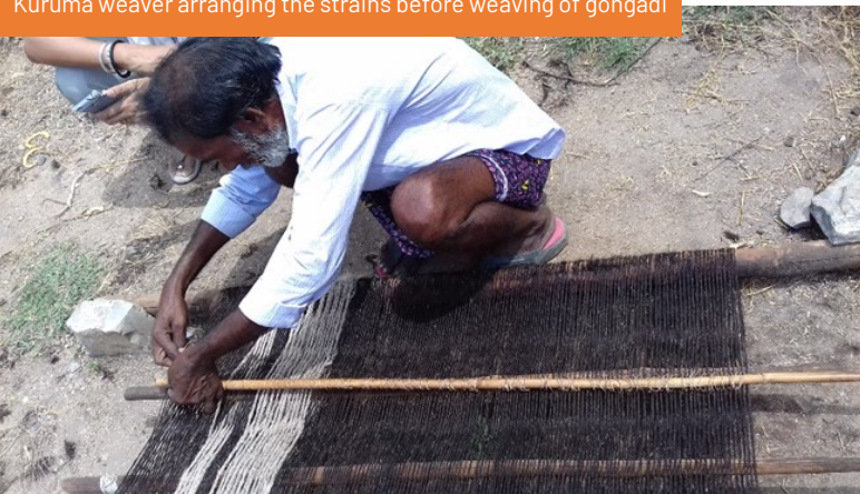
Kuruma weaver arranging the strains before weaving of gongadi
