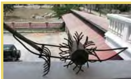
Photo 8.11 Simple weeder designed by Nong Sovann (Cambodia) with wooden axle, large nails, rake, and metal rods, costing less than USD 3.
