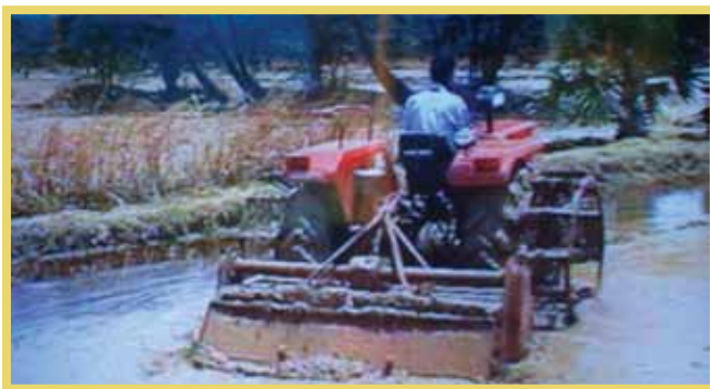
Photo 5.3 Puddling, rotovator-cum-leveler developed by a local mechanic-cum-farmer in Tamil Nadu
