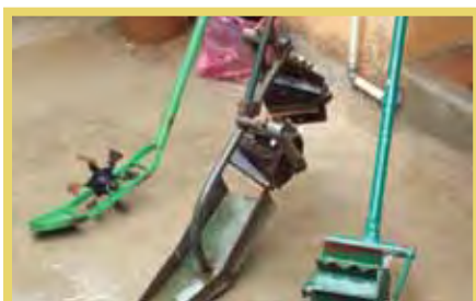
Photo 8.7 Rotary, cono and drum weeders
