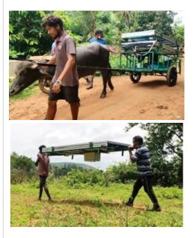
Energy Cart (new) - 2Hp pump & VFD, inverter & battery & Solar Pallaki -1Hp pump & VFD deployed on field
